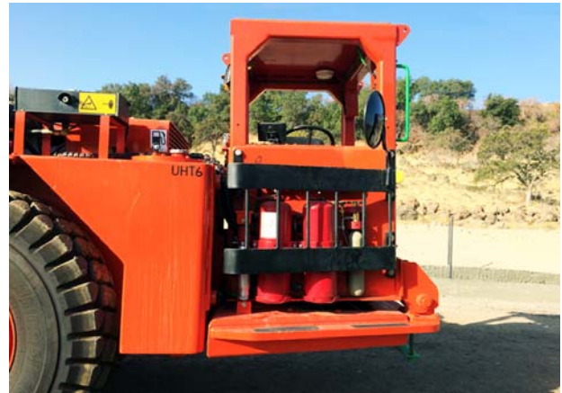
Suspension system installed on DUX model DT-20N with FOPS/ROPS canopy.
