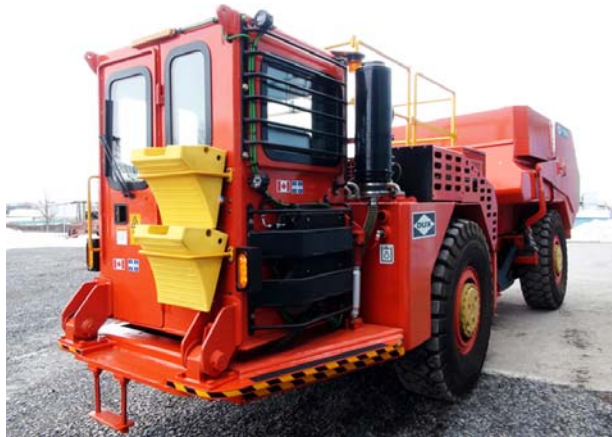
Suspension system installed on DUX model TD-18 with totally enclosed, fully equipped cab.
