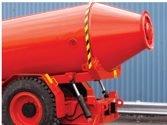
DUX S1-REMIX shown with optional drum lifting cylinders for adjusting the concrete discharge height as required.
