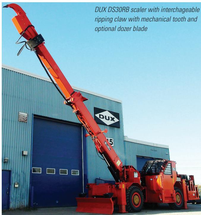
*DUX DS30RB scaler with interchangeable ripping claw with mechanical tooth and optional dozer blade*
