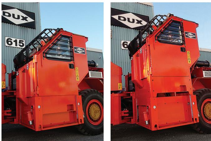
*FOPS comfort cab with hydraulic elevating feature*
