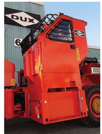
FOPS comfort cab with hydraulic elevating feature
