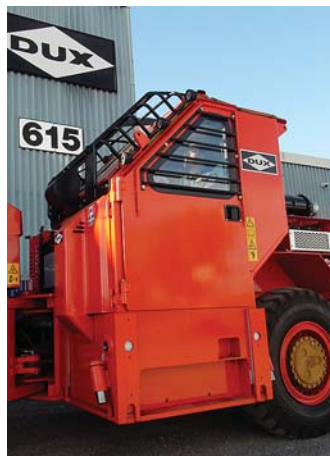
FOPS comfort cab with hydraulic elevating feature
