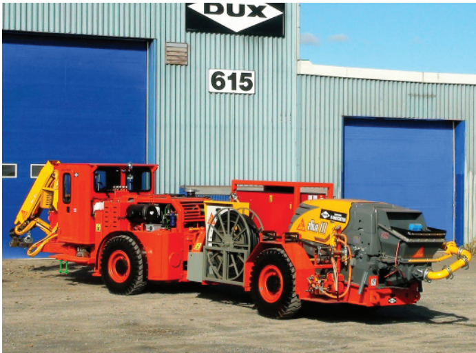
The DUX S1-Shotcreter with remote controlled robotic knuckle boom and piston pump
