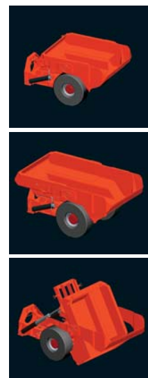
REAR LOADING BY SMALL SCOOP TO FILL RETRACTED FRONT
