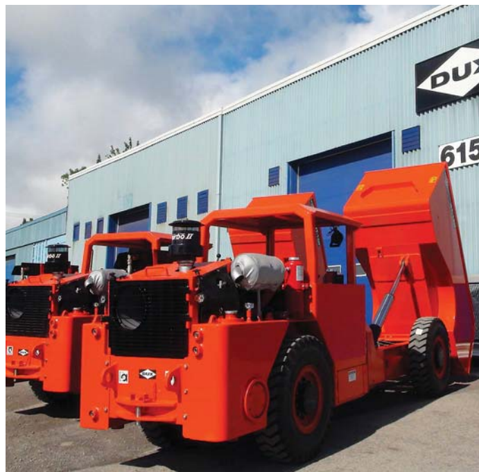
DUX DT-12N (narrow-version) measuring 1625 mm (5' 4") wide.
