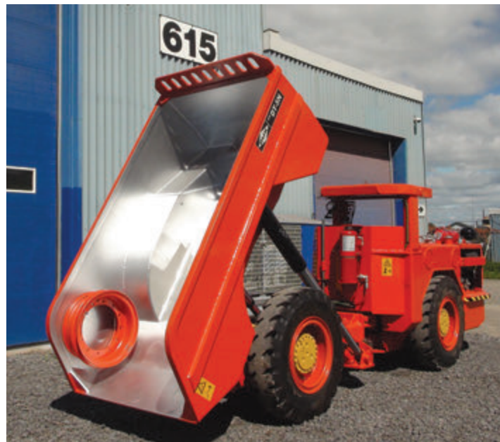
DUX DT-5N with optional FOPS/ROPS canopy and rapid clean discharge dump box with 60° dumping angle.
