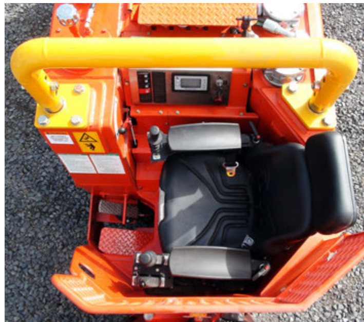
Operator side-seated for maximum visibility and bi-directional operation, heavy-duty adjustable suspension seat with arm rests and seat belt included.
